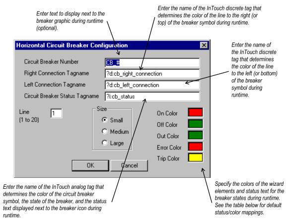
The breaker status values and the associated default colors are listed in the table below. Error status indicates that the breaker status inputs create an indeterminate state for the breaker.
